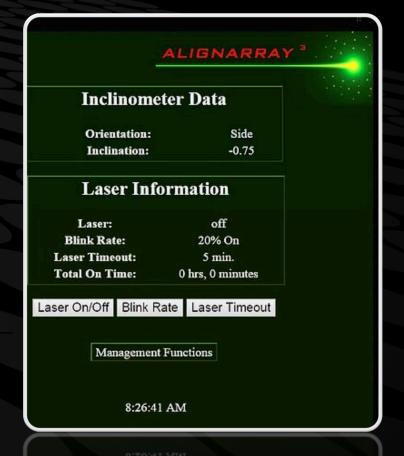
A Blinking laser can be easier to detect. Set desired blink rate and laser timeout.
