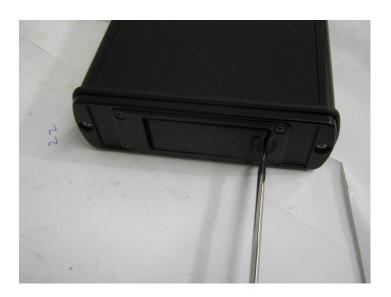
1) Place a small screw driver into battery bay door as shown. Gently push the blade at least 1/8" in.
