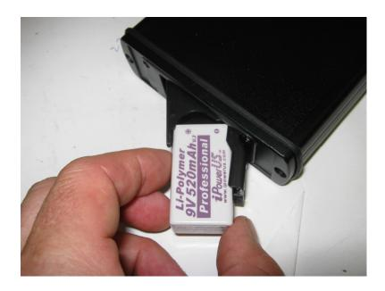
5) Slide the 9 V battery in with terminals in first, positive terminal closest to the outside (left side in picture).
