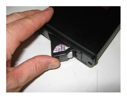
6) Close locking clip. Push battery bay back to the closed position.
